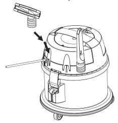
The inlet filter is in the lower part of the cover. It should be cleaned from time to time. If it is damaged it must be replaced with a new one.
