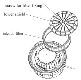
If the suction strength is reduced and cleaning of the filter does not help, the filter will have to be replaced with a new one!
