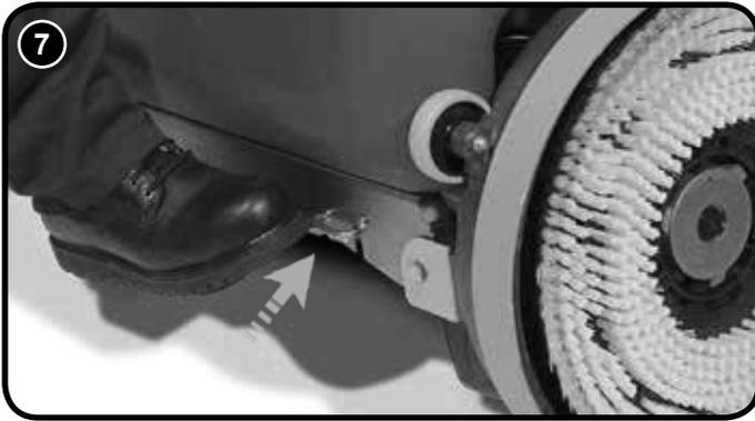
To tip the deck into the down position (Operating mode). Press in the brush deck locking pin (Fig.7) and rotate the brush deck (Fig.8).
