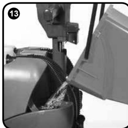
The large cap on the left can be removed for filling from a bucket or suitable container (Fig.13).
