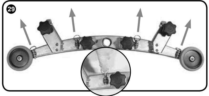
To clean the floor-tool, remove securing-pin and disconnect the lifting strap and remove the floor-tool securing pin pull-free the floor-tool from the rear of the machine. Rinse the floor-tool assembly with clean water and refit.
