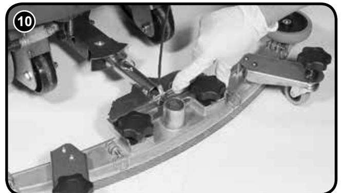
The lifting strap is held by a detent pin (Fig.10).
