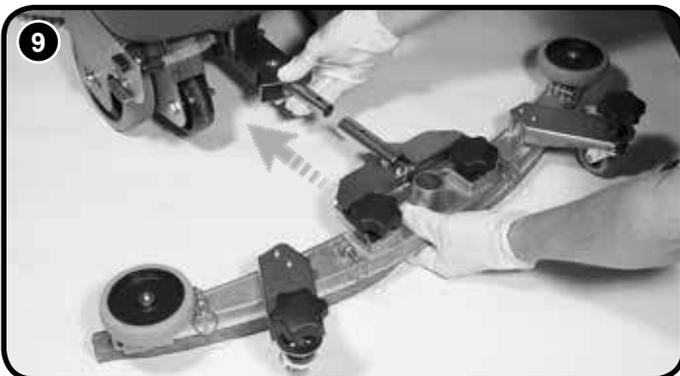
Fit the floor-tool and retain using the detent pin (Fig.9).
